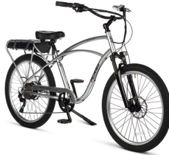
Class 2 Electric Bicycle Common power range: 250-750 watts or .333 to 1 horsepower (Pictured bike 500 watts) Maximum speed: 20 MPH
