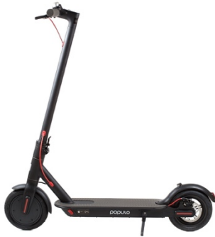
Electric Scooter Common power range: 250-500 watts or .333 to .667 horsepower Maximum speed: 15-20 MPH Distinctions to an electric bicycle: • No pedals for human propulsion • No seat, must be stood upon • Smaller wheels
