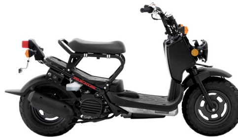
Scooter or Moped Common power range: 3 (50cc) to 20 horsepower (250cc) Maximum speed: 25-60 MPH Distinctions to an electric bicycle: • No pedals for human propulsion • More powerful motors • Faster maximum speed • Often combustion powered
