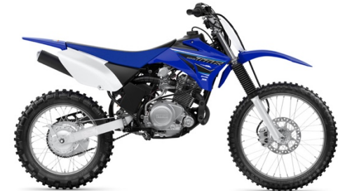
Off-Road Motorcycle/Dirt Bike Common power range: 6 (125cc) to 60 horsepower (450cc) Maximum speed: 45+ MPH Distinctions to an electric bicycle: • No pedals for human propulsion • Much more powerful motors • Much faster maximum speeds • Often combustion powered
